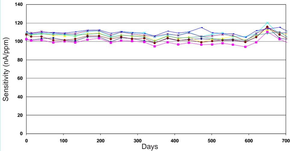
When sensors are tested monthly, their very good stability shows that they can be used in fixed sites, where maintenance and recalibration costs are important.
