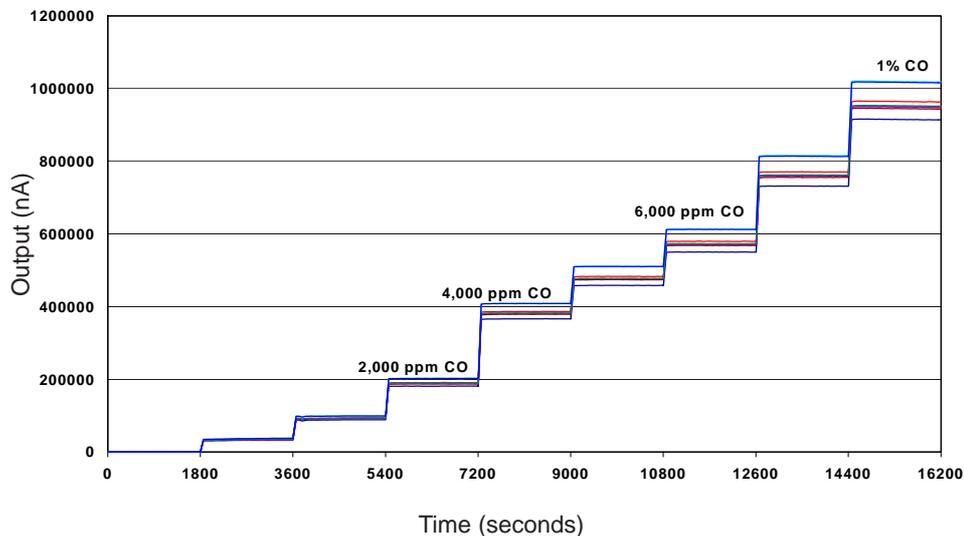
Figure 4 shows the response to step changes in CO concentrations from zero to 1% by volume.
