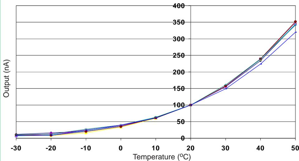
Hydrogen sensitivity is very dependent on temperature.
