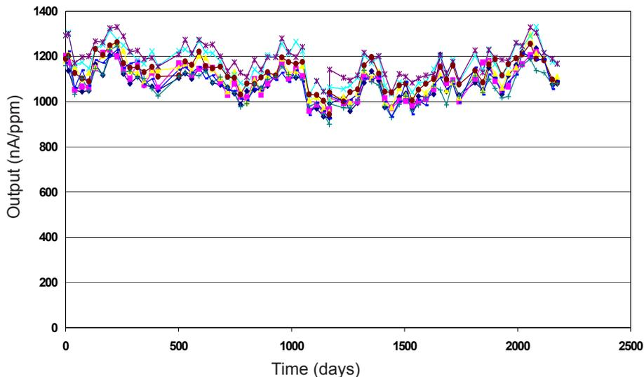
Figure 4 shows the excellent long term stability of the sensitivity of the H2S-AH resulting from the combination of patented design, superior electrochemistry and automated
