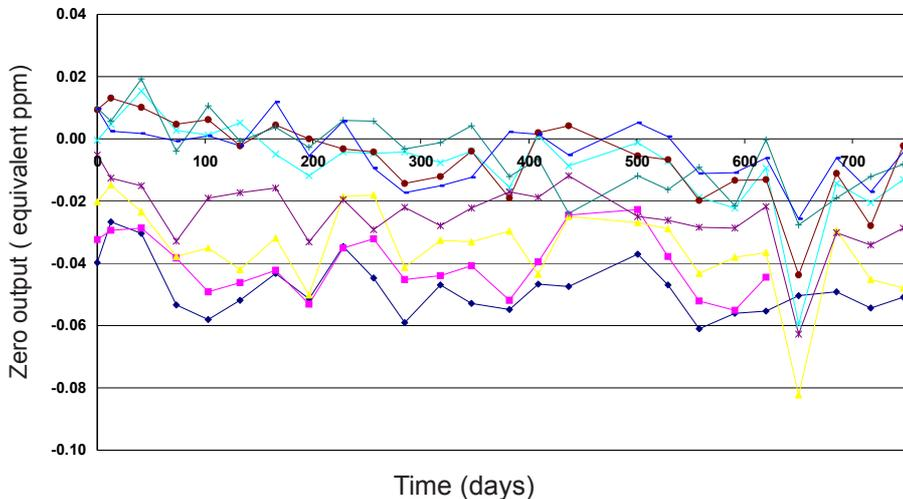
Figure 4 shows the excellent zero stability for the H2S-BH over 2 years, ensuring that low level alarms will remain stable.
