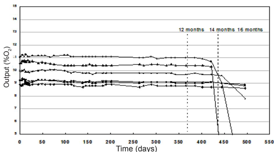
Figure 4 shows long term stability data for the O2-G1 sensors.
