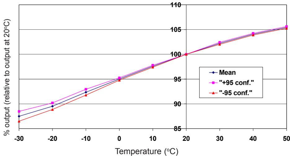
Figure 2 shows the variation of output caused by changes in temperature in 20.9% oxygen.
