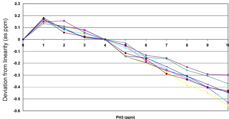
Figure 4 shows variation from linearity to 10ppm. Software correction between 0 and 0.5ppm can improve overall linearity.
