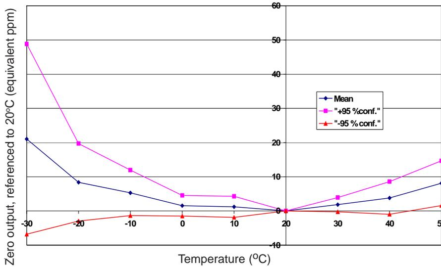
Figure 2 shows the variation in zero output caused by changes in temperature, expressed as ppm gas equivalent, referenced to zero at 20°C.
