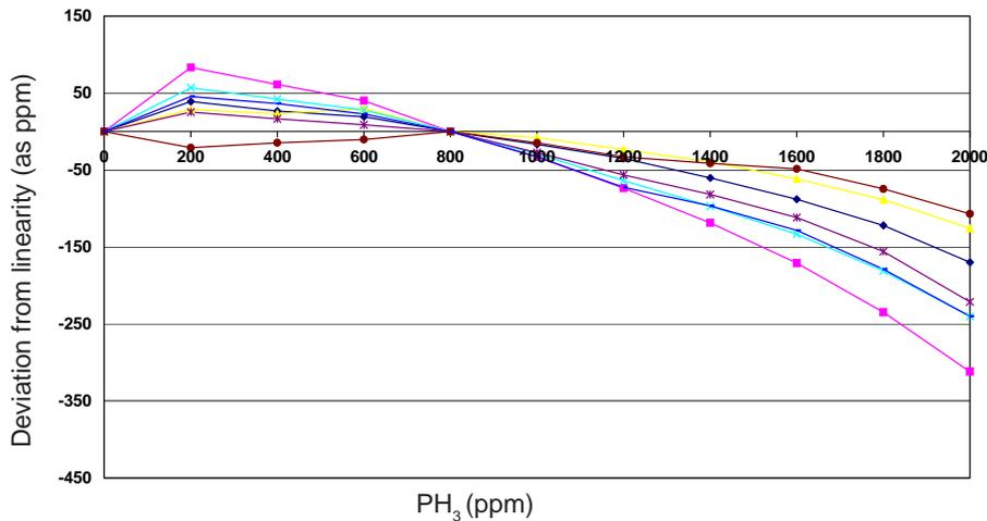
Sensor linearity is repeatable between sensors, allowing for software correction if required.
