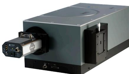
iDus 416 CCD mounted on a Shamrock 500i triple grating imaging spectrograph with silver-coated optics, ideal for low-light, high resolution NIR spectroscopy.
