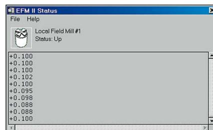
*EFM550 data can be displayed using optional Vaisala ALARM Automated Lightning Alert Risk Management Software to show current electric field measurements numerically and graphically*
