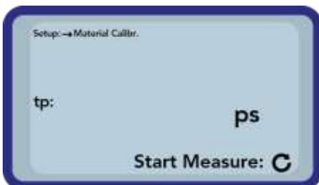
To start the measurement push the button „Measurement“
