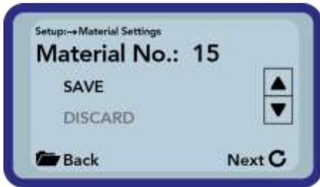
Finally you can store the calibration into the chosen calibration storage inside the probe. Choose „SAVE“ and confirm by pressing the button „Measurement“
