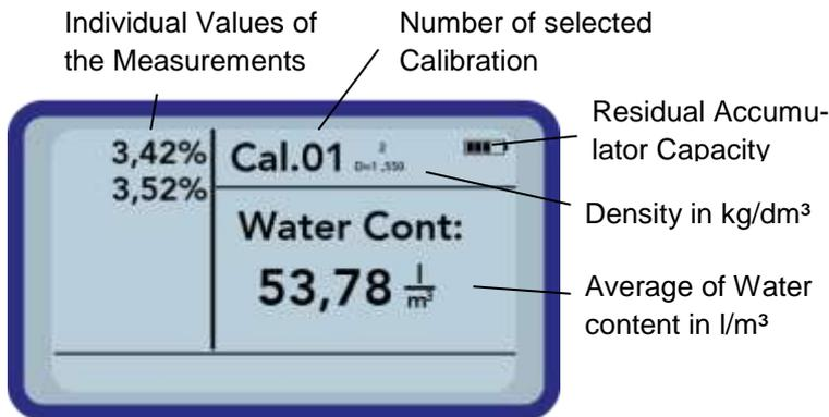
In order to delete the measurement series, actuate the button „Down“
