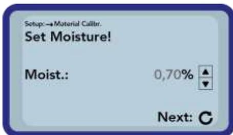
Next set the moisture of the material by pressing the buttons „Up“
