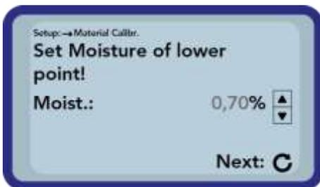
Next set the moisture of the lower moisture point by pressing the buttons „Up“
