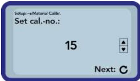
First you have to set the calibration curve to be changed (01 – 15) by pressing the buttons „Up“
