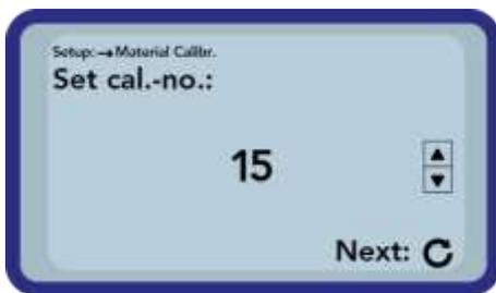
First you have to set the calibration curve to be changed (01 – 15) by pressing the buttons „Up“
