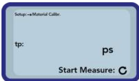
To start the measurement push the button „Measurement“
