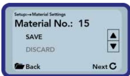
Finally you can store the calibration into the chosen calibration storage inside the probe. Choose „SAVE“ and confirm by pressing the button „Measurement“
