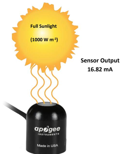
Example of total shortwave radiation measurement with an Apogee SP-214 pyranometer. Full sunlight yields total shortwave radiation on a horizontal plane at the Earth's surface of approximately 1000 W m<sup>-2</sup>. This yields an output signal of 16.82 mA. The signal is converted to shortwave radiation by subtracting the 4.0 mA offset and then multiplying by the calibration factor of 78 W m<sup>-2</sup> per mA.
