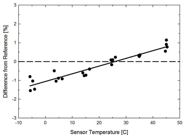
Mean temperature response of four Apogee silicon-cell pyranometers. Temperature response measurements were made at approximately 10 C intervals across a temperature range of approximately -10 to 50 C under sunlight. Each pyranometer had an internal thermistor to measure temperature. At each temperature set point, a reference blackbody pyranometer was used to measure solar intensity.
