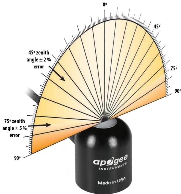
Directional, or cosine, response is defined as the measurement error at a specific angle of radiation incidence. Error for Apogee silicon-cell pyranometers is approximately  $\pm 2\%$  and  $\pm 5\%$  at solar zenith angles of  $45^\circ$  and  $75^\circ$ , respectively.
