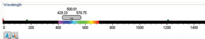
Wavelength drive: Sets the wavelength range for the current grating - drag slider to desired wavelength or just type in appropriate value
