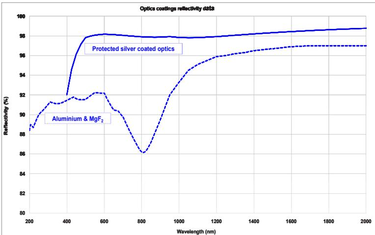
The graph shows the standard Al + MgF<sub>2</sub> optics coatings reflection efficiency versus wavelength.
