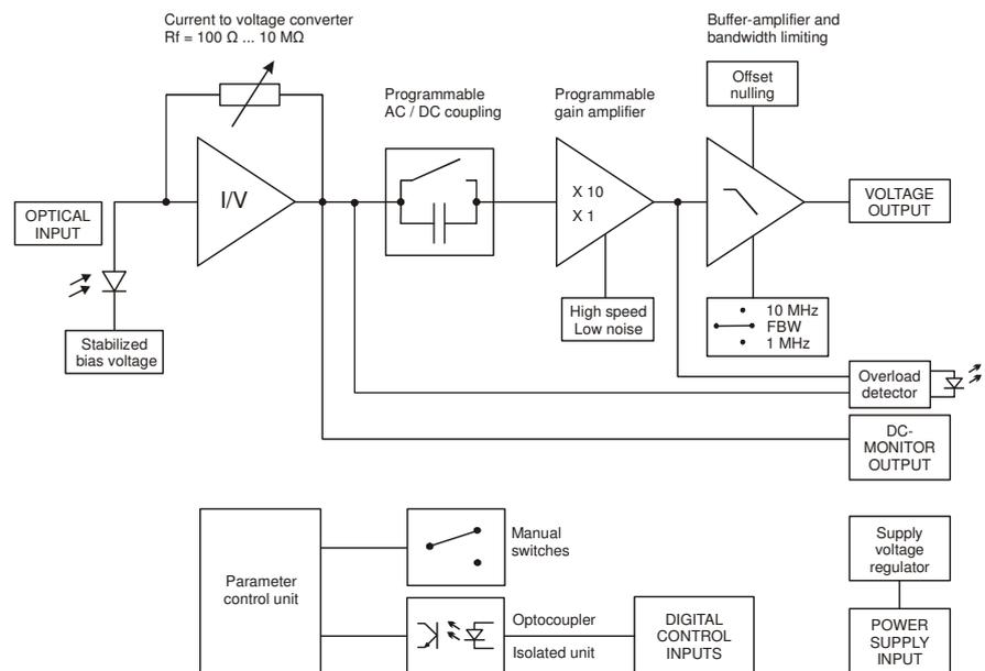
200 MHz Variable Gain Photoreceiver
