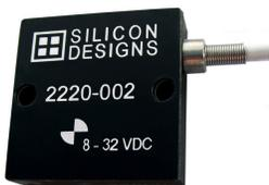
The SDI Models 2220 and 2276 are the high-performance versions of the 2210 and 2266, respectively. The 2220 and 2276 have an upgraded SDI accelerometer chip inside, reducing the bias and scale factor temperature shift performance and supporting greater temperatures from -55 to +125°C.
