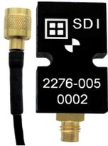
The SDI Models 2220 and 2276 are the high-performance versions of the 2210 and 2266, respectively. The 2220 and 2276 have the same upgraded SDI accelerometer chip inside as the 2470 and 2476, similarly reducing the bias and scale factor temperature shift specifications and supporting greater temperatures from -55 to +125°C.
