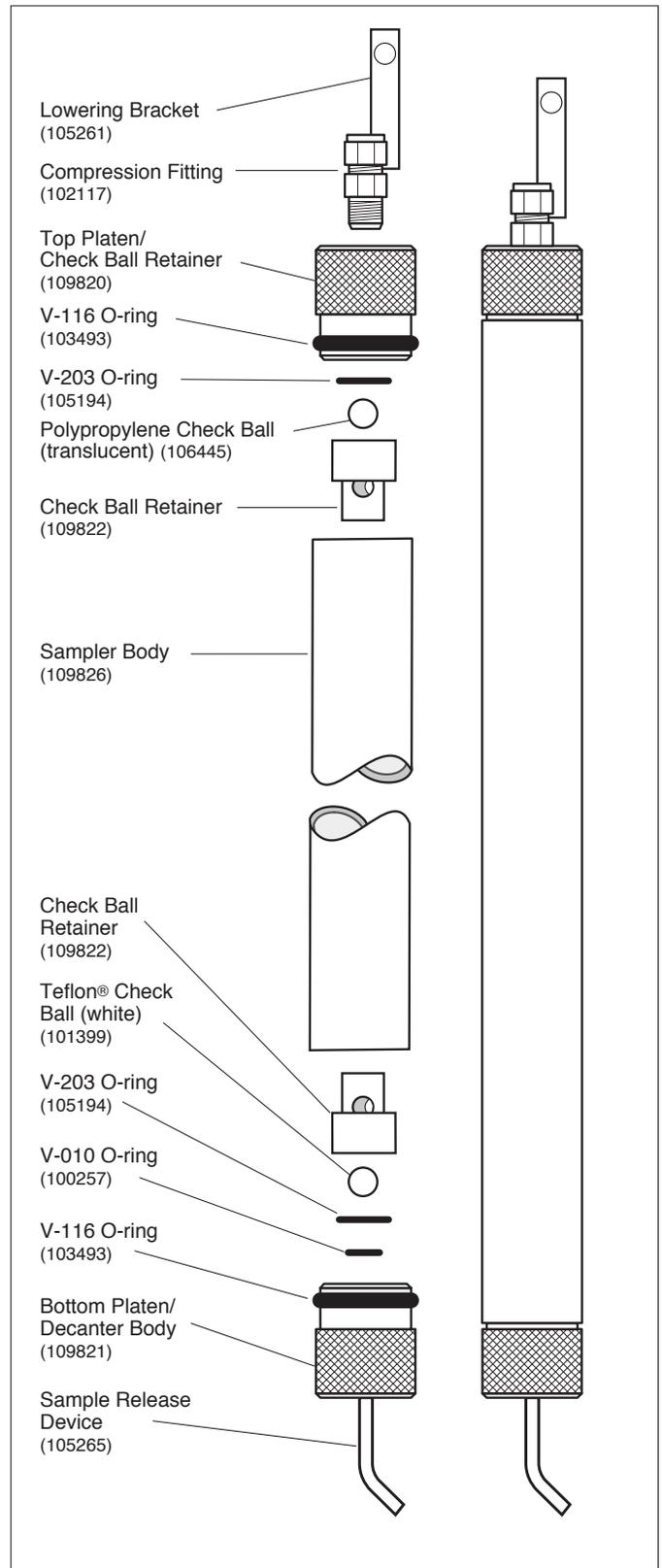
Model 425 1" dia. x 2 ft. Discrete Interval Sampler (109824)
