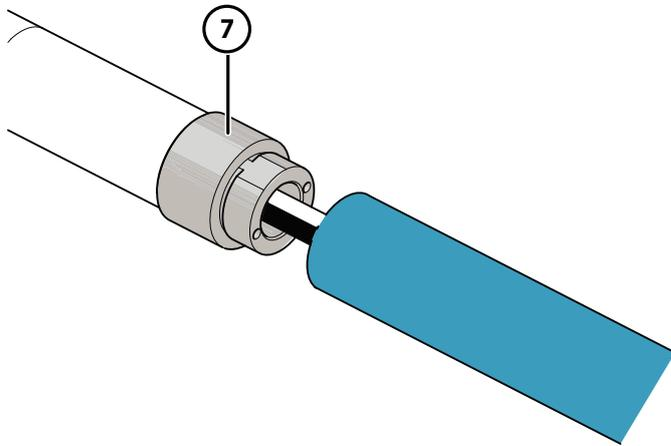
Figure 4 Supporting HMT330WPA with a Cable Conduit
